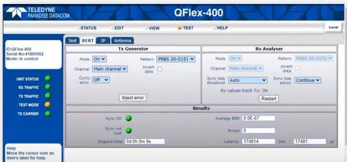
**Inbuilt Bit Error Rate Test Set (BERT):** The internal PRBS BER Tester allows pseudo-random bit patterns to be injected into the main traffic or overhead channel and the BER results to be monitored. Use of the ESC and AUX channels allows continuous real time traffic performance monitoring whilst the modem carries traffic. As well as average BER, number of bit errors and sync status, latency can also be measured.
