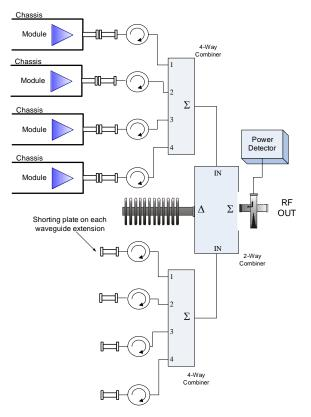
put power capability and gain will change as the number of active modules vary. The Outdoor PowerMAX system is designed with an Auto-Gain Control mode so that the overall system gain will remain constant in the event of a single module failure. See the table below.
